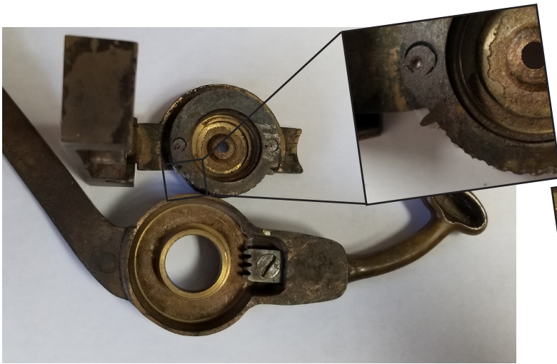
This is the window crank. Note how the gear on the top half has only two teeth left - the rest have been worn smooth.
